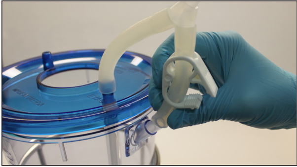
Figure 4. Attach clamp side of Y-tube to "CLAMP" port.
