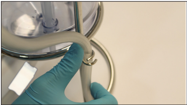
Figure 6. Secure fluid evacuation tube in pigtail hook.
